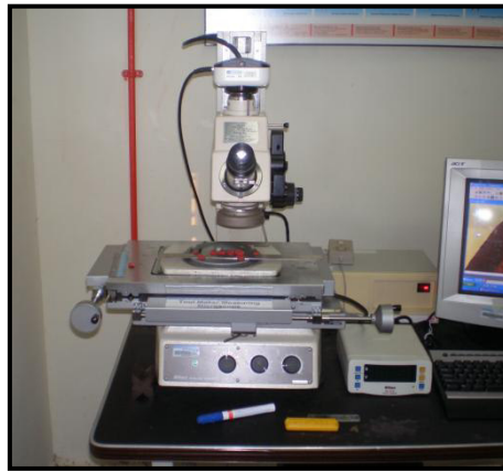
Figure 2.5: Nikon Toolmakers Microscope
