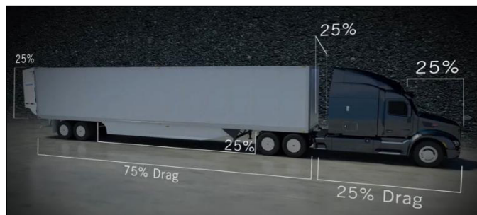
Figure 1.7: Drag Force Loss Percentage Rate
