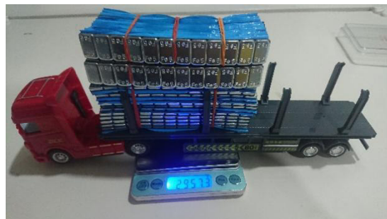
Figure 3.11: Trellar With A Weight Of 4 295.73g On The Front
