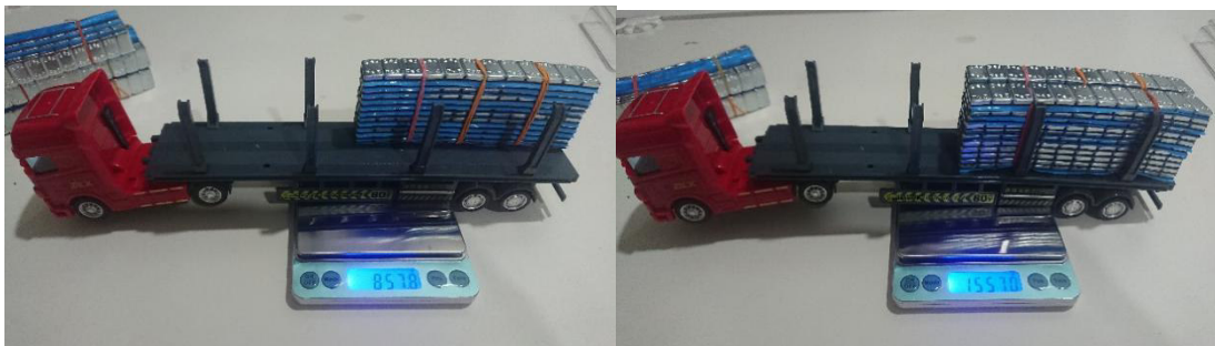
Figure 3.14: Trellar And Weights 1 700g And Weights 2 1400g On The Back.
