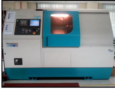
Figure 2.4: Power Path CNC Lathe Machine 15
