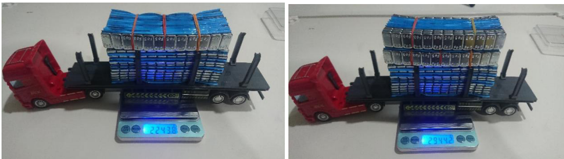
Figure 3.13: Trellar And Weight 3 2100g And Weight 4 2800g In The Middle.
