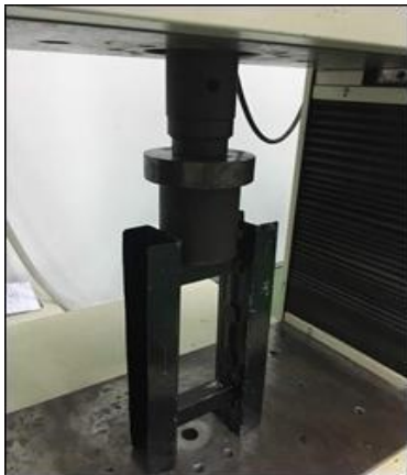
Figure 4.9 Compression Strength Test on Joint of C-Channel Trusses Holder
