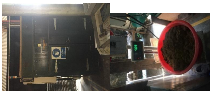
Figure 5: Dry finely crushed EFB in the oven and weight according to the specification
