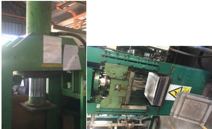
Figure 7: Put the molded mixture in the cold press machine and then hot press machine at 185°C and 90/3, 70/2, 50/1 (pressure/minute)
